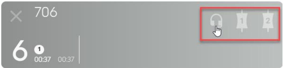
SELECT HEADSET OR DEVICE 1 OR DEVICE 2, AS NEEDED. HEADSET BEING SELECTED IN THIS EXAMPLE
